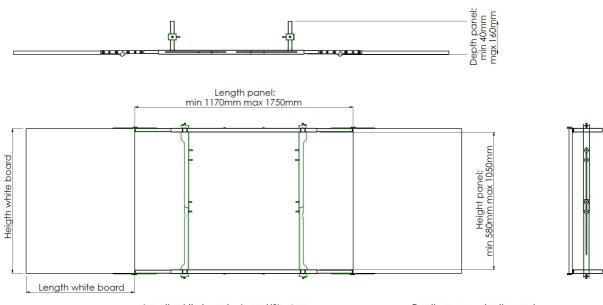
Length white board = (panel/2) - 4mm Heigth white board = Height panel + 47mm Depth open = depth panel Depth closed = depth panel open + 30mm
