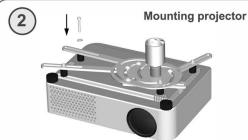
Mount the projector to the arms. Use the supplied spacers, bolts and washers. In case of a height difference between the mounting points and the projector, spacers could be used to intercept this difference. Position the ball joint above the centre, or at the nearest possibility of the projector lens.
