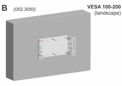
Mount the connecting plate at the back of the screen using the VESA 200-100 mounting holes (landscape). Use the supplied mounting material.
