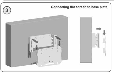
Attach the connecting plate to the base plate.
