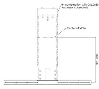
Can also be used above screen, by turning bracket upside down
