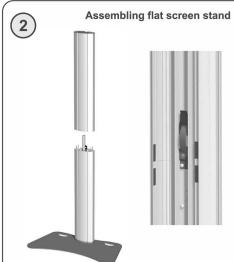
Assemble the flat screen stand (see mounting instructions flat screen stand). Assemble only the column(s) on the floor plate. The head of the stand wil be positioned later on.
