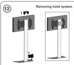
Untie the winch strap by turning back the winch. Unhook the strap. Remove the hoist guide and the winch from the flat screen stand (only the hoisting plate and the mounting bars remain attached to the flat screen stand). After the cables are connected, the head of the stand can be secured with the securing profile and an optional lock (see installation instruction flat screen stand).
