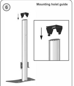
Slide the hoist guide into the top of the column by using the T-ducts. Tight the knobs to fix the hoist guide.
