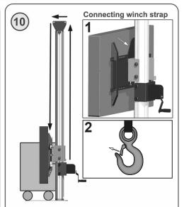
Connect the winch strap to the hoisting plate at the back (1), make sure the hooks safety latch is closed (2) and tighten the strap by using the winch.
