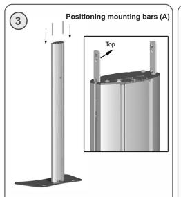
Slide in both T-ducts of the column a mounting bar. Be sure the right side is on the top (see picture). Slide them carefully down towards the floor plate.
