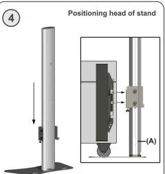
Slide the head of the stand from the top downwards by using the T-ducts on both side of the column. Position the head on the right height. This is the height where the three coupling boxes at the back of the flat screen fit into the slots of the head (when the flat screen is positioned in the flight case). Tight the knobs to fix the head.
