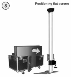
Remove the cover of the flight case. Open the door of the flight case and roll the case towards the flat screen stand. Make sure the three coupling boxes behind the screen fall into the slots of the head of the stand.
