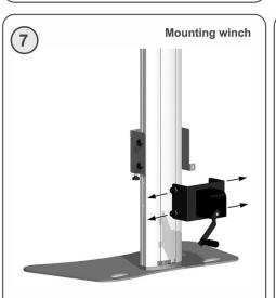
Pull out the four knobs of the winch bracket. Turn the knobs to fix them in their outer position. Mount the winch to the column by shooting back the knobs into the holes of the mounting bars.
