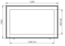
The standard dimensions A & B can be replaced by custom values.
